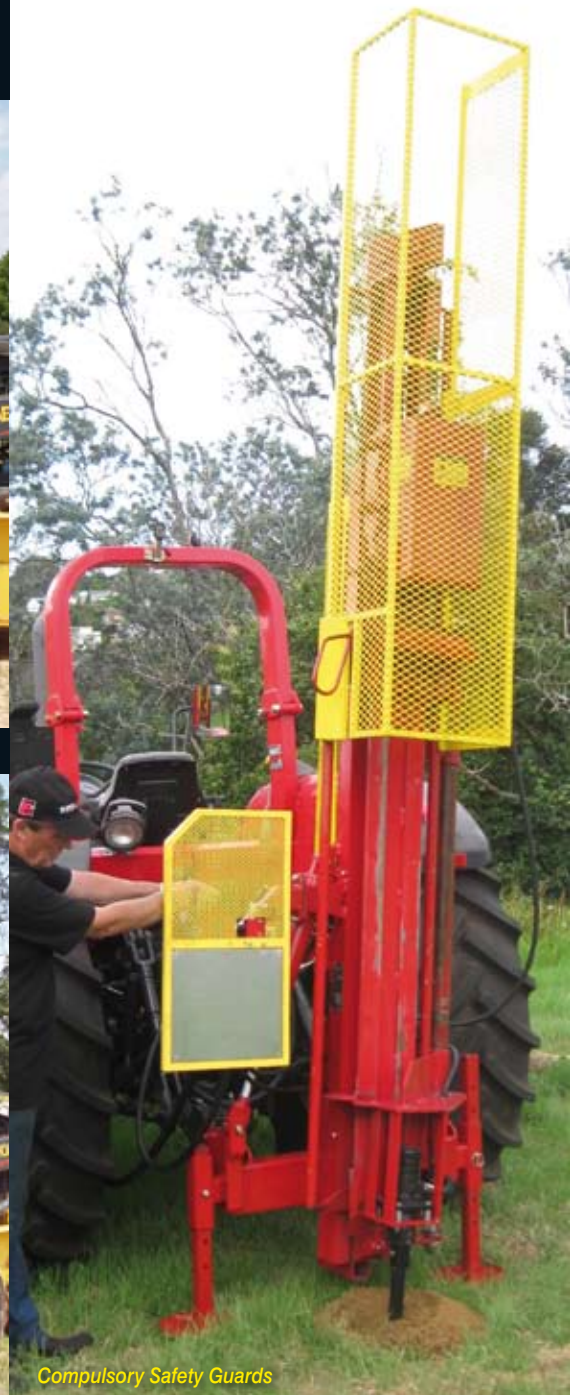
Series II Expander Rear Mounted with Guarding & Auger
