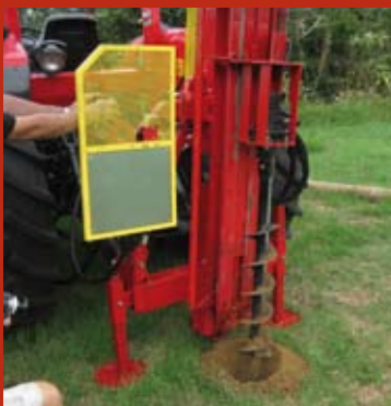
Series II Expander with Compulsory Safety Guarding & Auger
