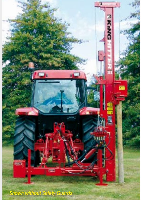
Series III Side Mount - 450mm side movement
